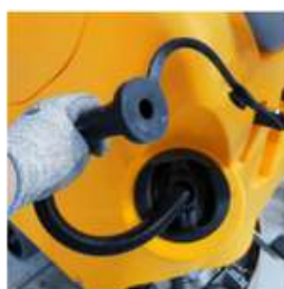
Cap with hose for the water loading
